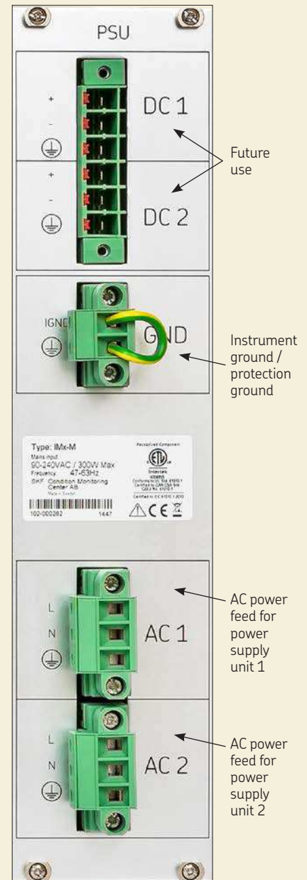
Power Supply input connector board (part of backplane) (rear view)
